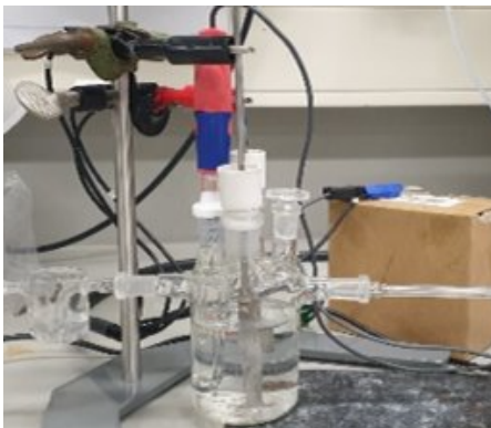
Figure 1. Three-electrode cell setup for electrodeposition
