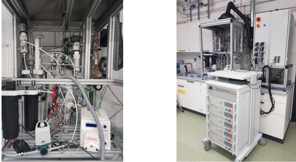
Figure 1: Single cell test bench "BEAST" at HyCentA, with the cell conditioning infrastructure shown on the left image and the Toellner 4 quadrant multipliers with the Gamry LPI 1010 on the right image.
