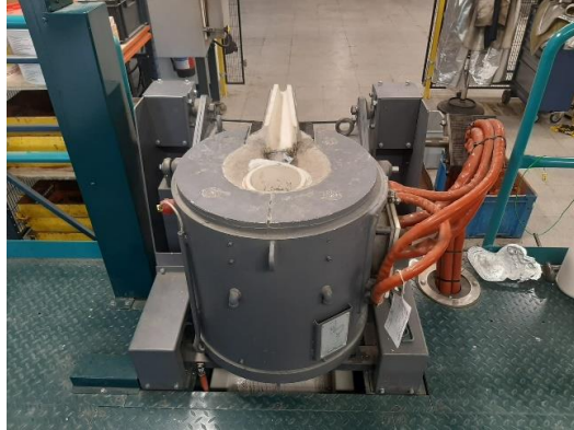
Figure 2. Oven used to produce the target CoCrCuFeMnNi alloy under Ar atmosphere.
