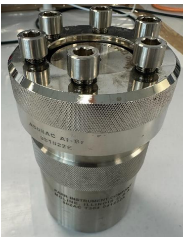
Figure 1 - hydrothermal reactor for synthesizing catalyst
